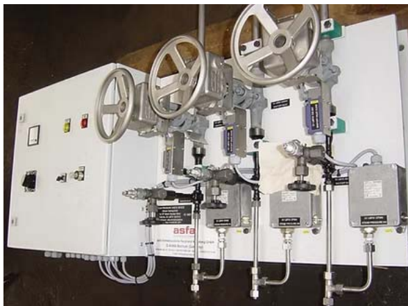
Steam testing unit with a rack for wall mounting Execution with mechanical pressure switches
